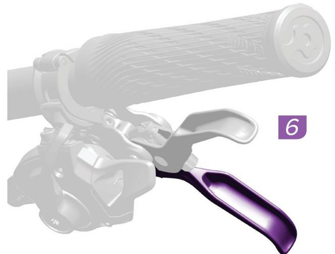
Pull the brake lever to the handlebar, tighten the caliper bolts to 9-10 N·m (80-90 in-lbs), then release the brake lever.
