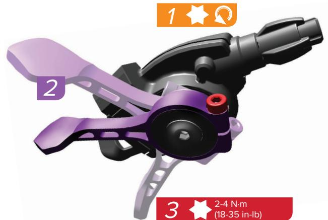
Loosen the reach adjust bolt to adjust the shift paddle to the desired angle, then tighten the bolt to 2-4 N·m (17.7-3.4 in-lb).
