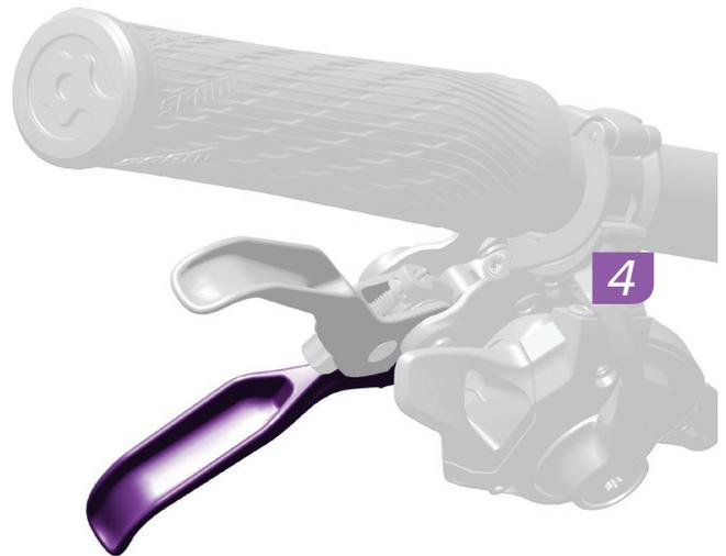
Pull the brake lever to the handlebar, tighten the caliper bolts to 9-10 N·m (80-90 in-lbs), then release the brake lever.
